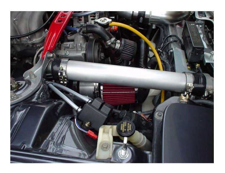
Blitz FMIC inlet neck was cut off, inverted, and rotated CC.
