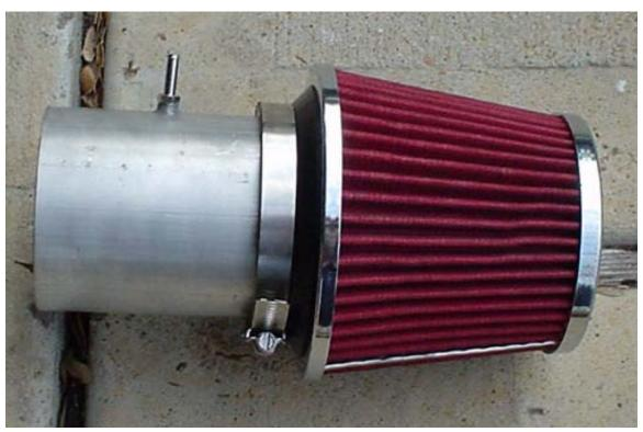
The extension pushes the air filter closer to the radiator. My stock coolant hose was in the way because my Blitz FMIC causes the radiator to sit back further than stock. You might not have this problem. I had to cut off the angled end of the radiator inlet pipe, and make a special coolant hose using a COOL FLEX kit. It gives a great amount of clearance.
